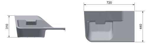
Figure 6. Overall dimensions of the WHBV-101W-RH-NB.
